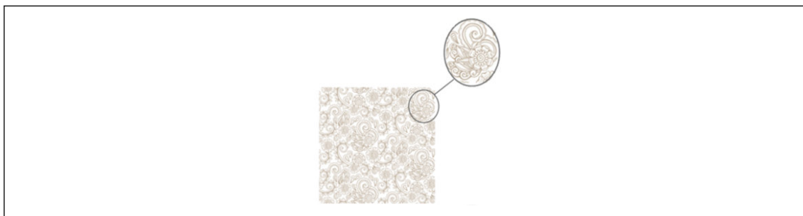
Example of an acceptable magnified view filed as a separate view
